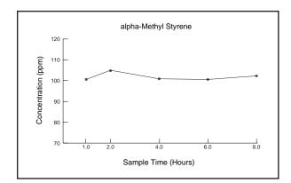
The mean sampling rate was 12.3 ml/min (3.57 mg/ppm/hr) and was calculated as a weighted average of the 1, 2, 4, 6, & 8-hour exposure periods based on a mean concentration of 98.9 ppm.
