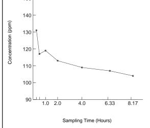
The mean sampling rate was 9.8 ml/min (3.33 µg/ppm/hr) and was calculated as a weighted average of the 1, 2, 4, 6, & 8-hour exposure periods from these results combined with those of the 575-002 sampler based on a mean concentration of 103 ppm.
